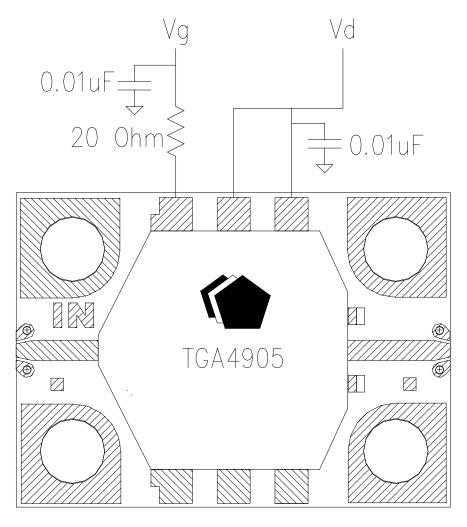
Two 1 mil wires are recommended for the RF Input, RF Output, Vg, and Vd1. Six bondwires are recommended for Vd2.
